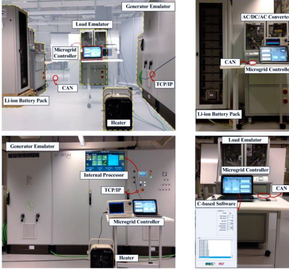
Figure 13. (a) Experimental setup for the implementation of the test grid including (b) a generator emulator, (c) a Li-ion battery pack, and (d) a load emulator.
