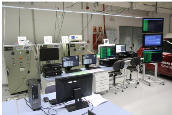
Figure 10. Overview of the microgrid: microgrid emulators (back), electric vehicle (right) and data acquisition and control system (front).
